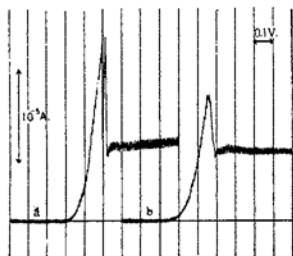
Fig. 1.—Polarograms of p - and o -nitroanilines in the supporting electrolyte containing no gelatin; (a) p -nitroaniline ( 0.5 \times 10^{-3} M ), (b) o -nitroaniline ( 0.5 \times 10^{-3} M ). Each polarogram begins at -0.4 volt vs. N. C. E.
